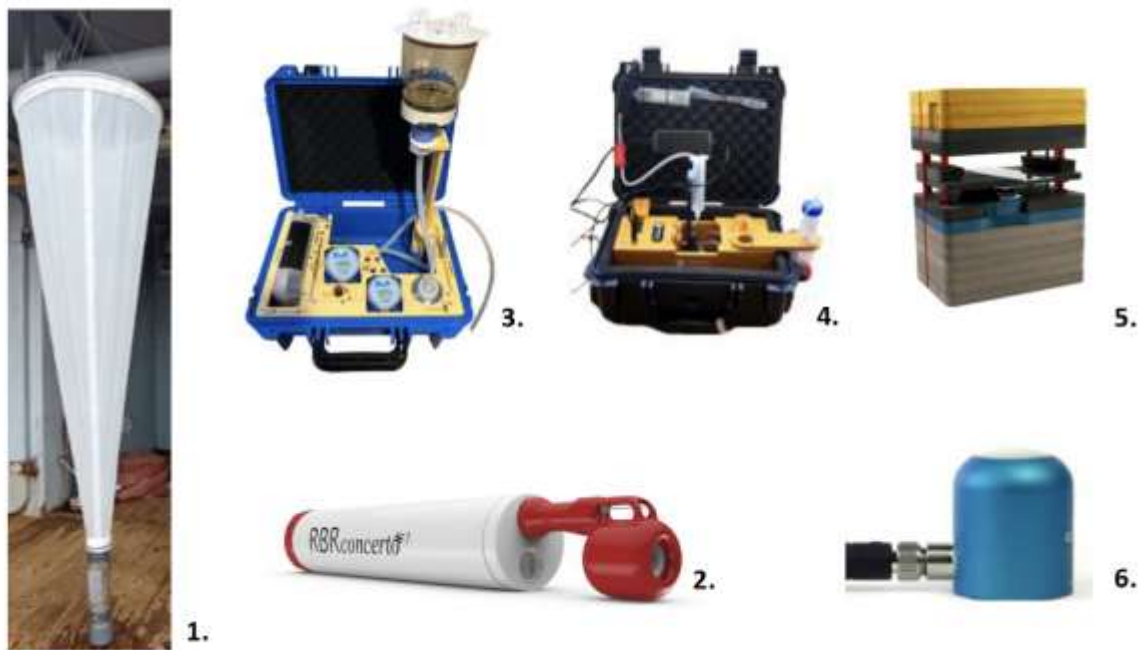
Figure 1. The innovative ‘P2-Bougainville’ kit for frugal oceanography. 1. 20- \mu\text{m} and 50- \mu\text{m} nets: plankton nets with specific mesh sizes deployed at each sampling station, either vertically or horizontally. 2. CTD probe: a commercial probe equipped with sensors measuring conductivity (salinity), temperature, and depth during each deployment at a sampling station. 3. Lamprey: a portable mini-station for filtering planktonic biomass, equipped with a 47 mm diameter membrane filtration funnel connected to a peristaltic pump. 4. PlanktoScope: a portable, semi-continuous flow microscope designed for quantitative imaging (counting, measuring, classification) of planktonic organisms and particles between 50 and 200 \mu\text{m} . 5. Curiosity microscope: a compact and user-friendly digital microscope with four magnifications (x2, x5, x10, x20), allowing semi-quantitative observation and imaging of plankton (organisms between 10 and 2000 \mu\text{m} ). 6. PAR sensor: sensor for continuous measurement of Photosynthetically Active Radiation.
